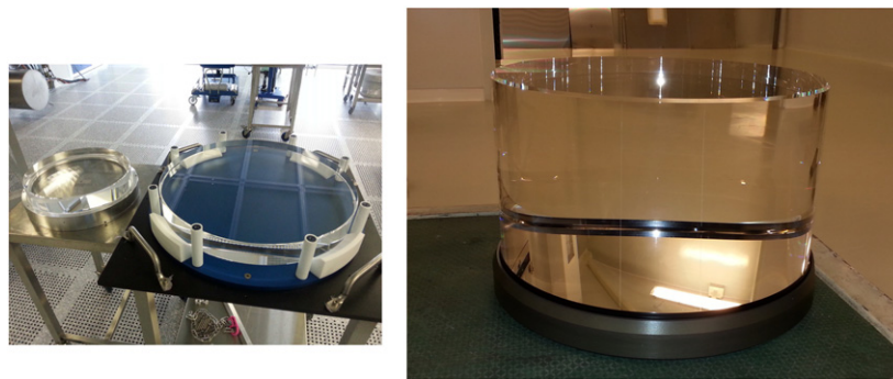
Figure 4. Left: PR substrate (35 cm in diameter, left) beside the large BS of 55 cm. Right: a test mass.
